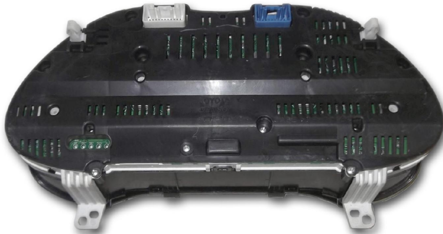
Fig.4. Bottom side of the instrument panel with connectors
